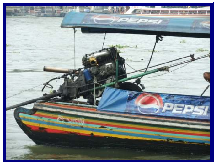
Long tail boat utilising a lorry engine
